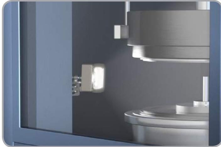
WLC90 heavy duty LED light withstands high temperatures and other hazards to illuminate an enclosure on rubber injection mold machinery
