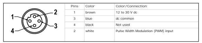
For maximum intensity, leave the white and black wires floating or connected to common.
