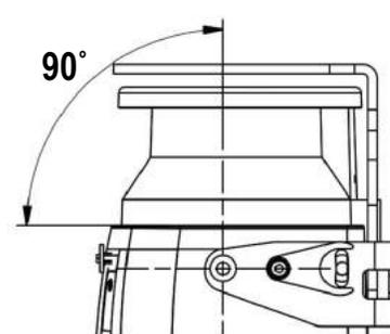
Figure 3. Adjust the scanner angle
