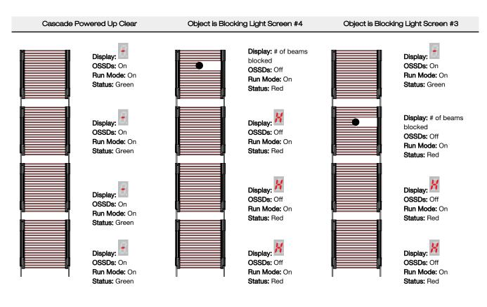
Figure 41. Cascade Indicator Status Conditions
