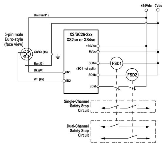
Figure 38. Generic Wiring Diagram—XS/SC26-2 Safety Controller
