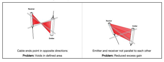
Figure 18. Examples of Incorrect Emitter/Receiver Orientation
