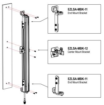
Figure 21. Mounting the center- and side-mount brackets
