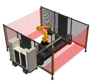
Figure 42. Light screens guarding a robotic cell
