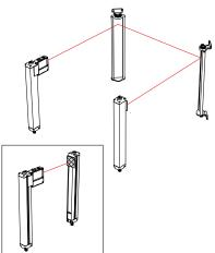
Figure 27. Optical alignment using the LAT-1-SS
