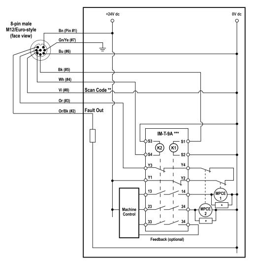
Figure 40. Generic Wiring Diagram—IM-T-9A Interface Module (1-Channel EDM)
