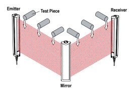
Figure 31. Trip Test with Corner Mirror
