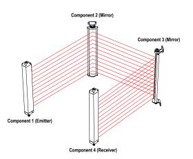
Figure 28. Corner Mirror Alignment
