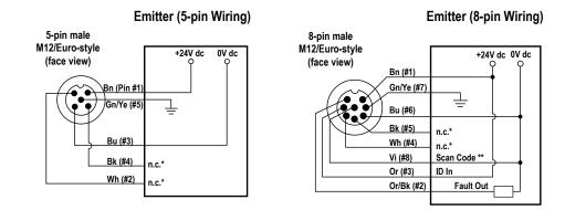
Figure 35. Generic Wiring Diagram—Emitter
