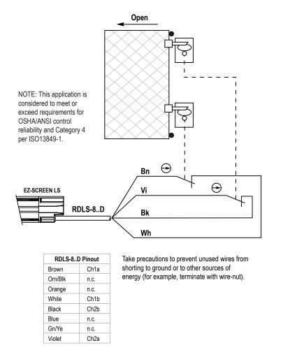
Figure 47. Monitoring two positive-opening safety switches
