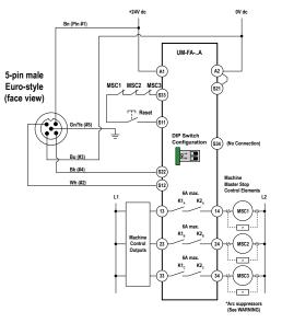
Figure 36. Generic Wiring Diagram - UM-FA..A with Auto Reset
