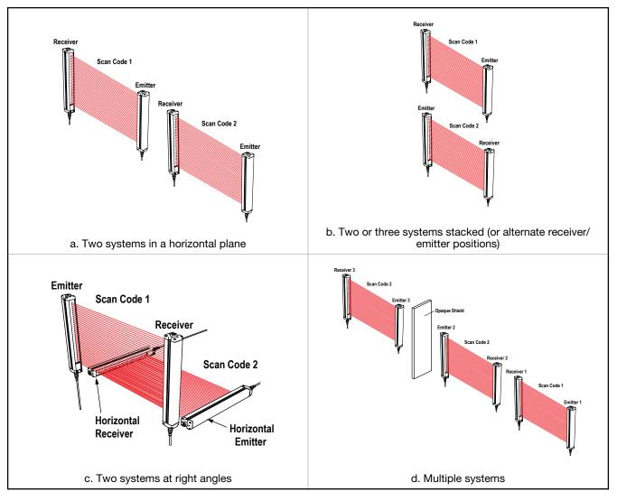
Figure 19. Installation of Multiple Systems
