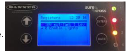
DXM Controller Display. The green LED indicates all level measurements are between the threshold settings. The amber
