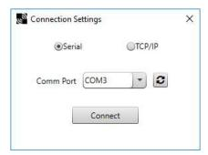
If multiple comm ports are visible, try each one until the software is able to connect to the device.
