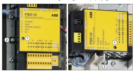
3. Make sure that the FSO data cable (terminal X110) is connected to the drive.
